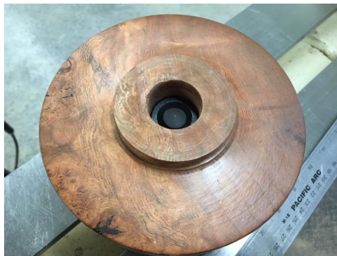
I use a dowel to turn the light on and off by inserting the dowel through the headstock spindle and pushing the button as pictured below.
